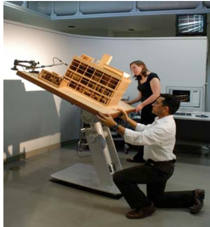
Analysis of an architectural model using the heliodon, which simulates sunlight penetration and shading at different times of day and during different seasons
